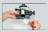
For cleaning and disinfection, remove both the transparent Breath Shield and the mounting clip from the instrument.
