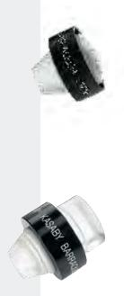
Barraquer Tonometers are based on Maklakov's principle of applanation tonometry. By direct corneal contact, the meniscus ring can be compared to determine intraocular pressure.
