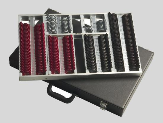
The **<u>Corrective Curve Trial Lens Set</u>** is designed and manufactured on a base curve allowing for thickness and space between stacked lenses. Each trial lens is mounted into an aluminum holder of uniform size; and the lens area is relative to the power of the lens. This stackable feature and the corrected curve fabrication is the main benefit of this type of trial lens set.
